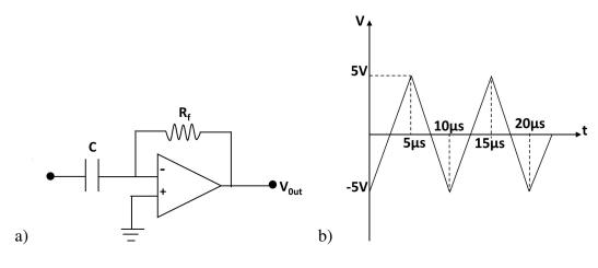
determine the output voltage waveform.
